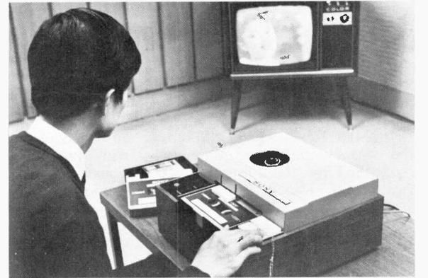
THE SONY Videocassette player is a simple, compact, easy to operate unit. Loading and unloading is a one-hand operation, left. The prerecorded programs are screened through any standard television set, color or black and white, right, by attaching it to the antenna base.
