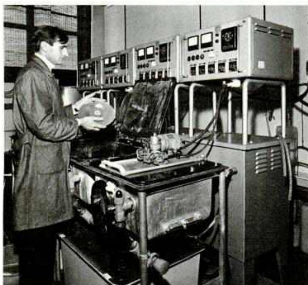
The electro plating system used for the production of metal parts to press records.
