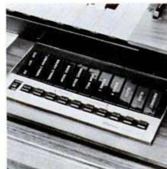
THOMAS ORGAN CO. reports that it sells more than 70 per cent of its organs with built-in Band Box, a versatile rhythm unit designed especially for electronic organs. The unit features 10 voices: crash sycmbal, brush cymbal, bass drum, snare drum, drum roll, bongo I, bongo II, block, clave and castanet.
