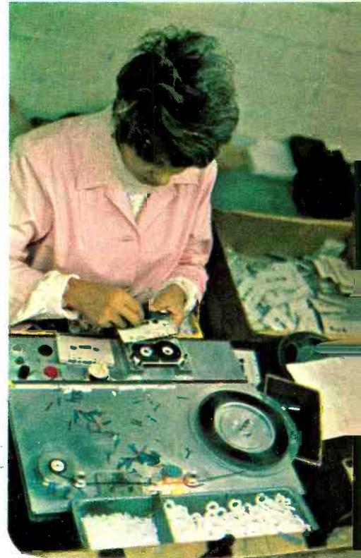
Lines of slit tape are fed onto spools (left) before moving to the loading and assembling process (above) where girls feed the tape into plastic cases.
