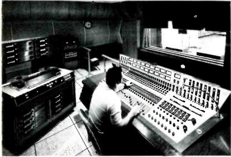
RCA's new Chicago recording center features an ultramodern control room with a 16-track console.
