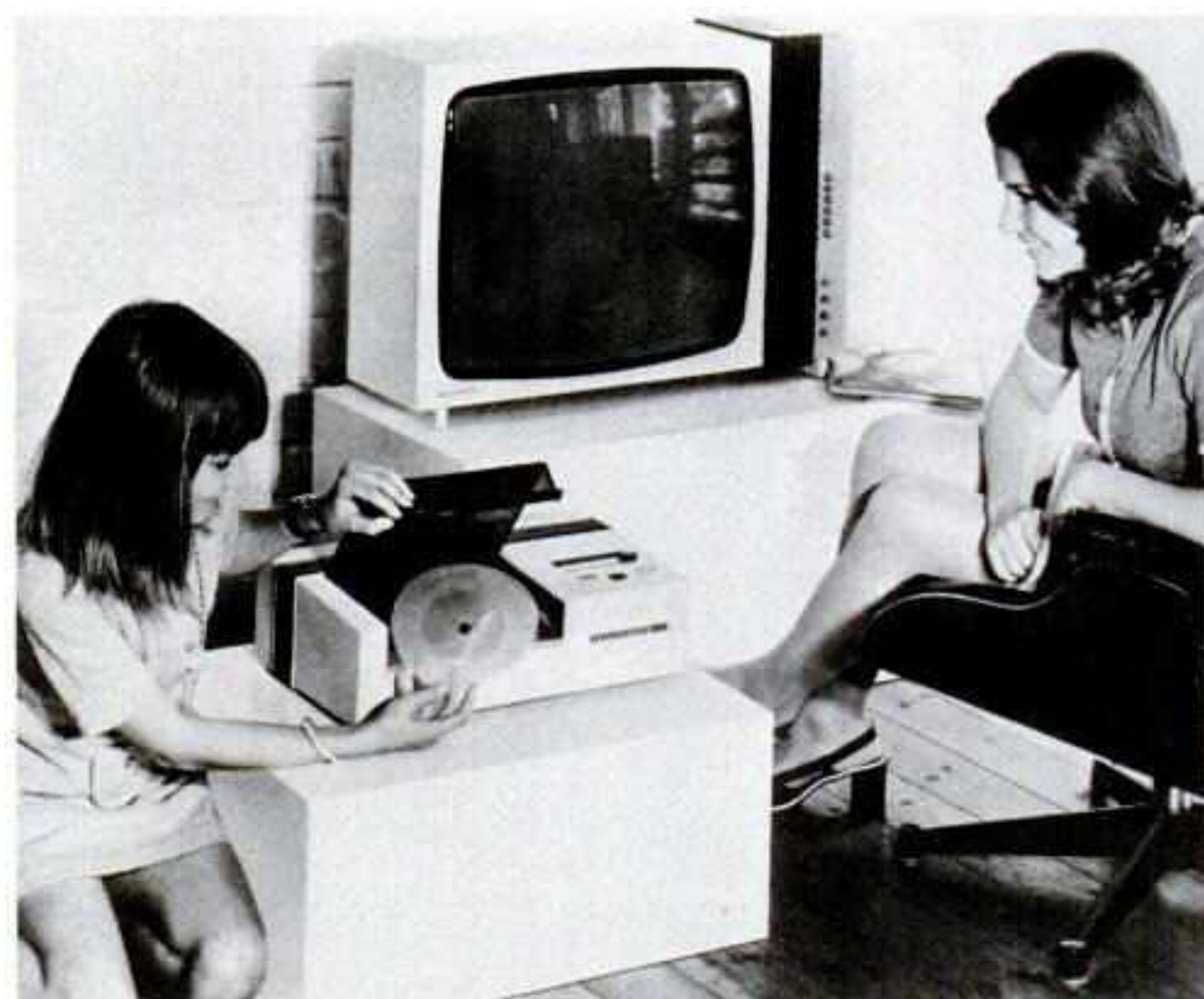
BY THE development of a new vertical recording method (top), it is possible to cut between 130 and 150 grooves per millimeter. The video disk player is child's play to operate (bottom). Repertoire will range from entertainment to news.
