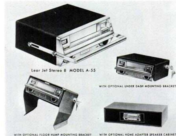
AUTO players now move from the car into the home such as this Lear Jet Model A-55. The unit mounts and locks under the dash or over the transmission hump and has a speaker enclosure for home use. The basic unit lists for \$69.95.
