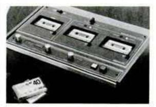
WOLLENSAK/3M Co. offers compact cassette duplicator Model 2770 for suggested list price of \$995. Duplicator makes two copies of a C-30 cassette simultaneously from one master in less than a minute.
