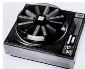
TELEX Model 48-D automatic stereo tape cartridge changer with pre-amplified deck switches and selects 12 8-track cartridges of any length in four operation modes. Listing at \$249.95, changer operates vertically and horizontally. Spare rotary magazines are available.
