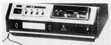
GE'S TA640 8-track tape deck, retailing for \$219.95, plays all 4-channel prerecorded tapes through 2-channel system. Among other features are two microphones and a one/all switch to allow recording on one track or all four in sequence.
