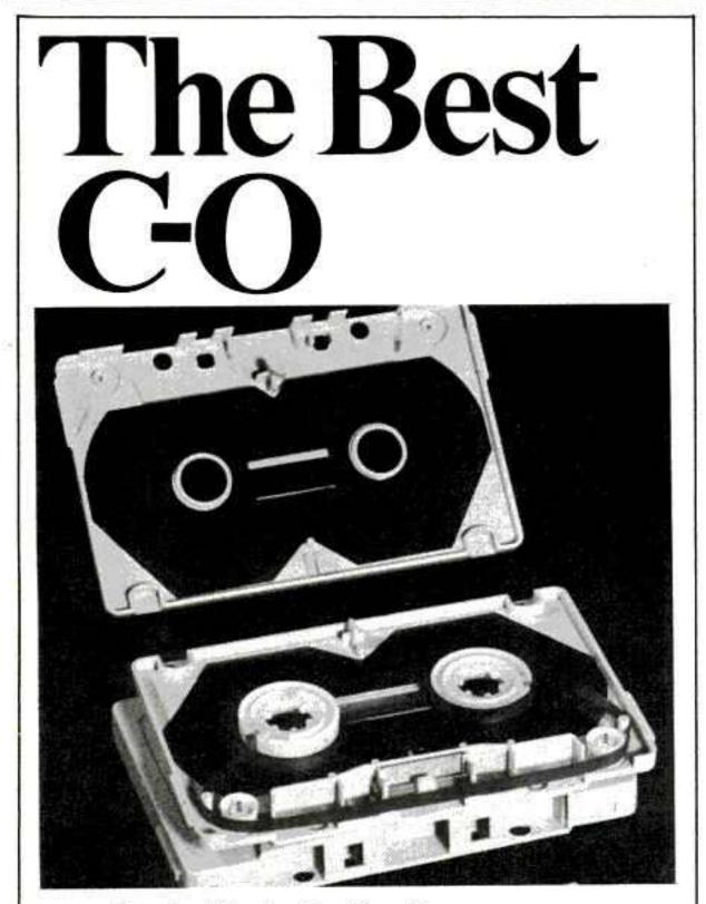
Standard Norelco Configuration Leader loaded Acetal hubs and rollers Graphite-coated Mylar washers Precision machined, stainless steel pins M-36 silicone zinc-plated shield Bi-axial oriented styrene window High heat, medium-impact polystyrene shells Windows and shells sonically welded Phosphor bronze spring pad Standard shell colors: black, grey or white Available tabs in or out
