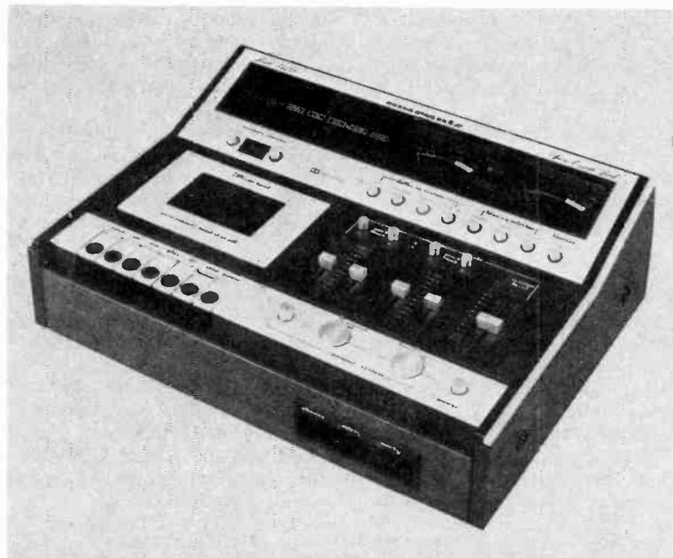
**MORE THAN** a stereo cassette deck, the Marantz model 5420 offers four-channel mixing with pan pots, Dolby noise reduction and cassette recorder with ferrite heads. Top loading unit has three-position tape bias switch.
