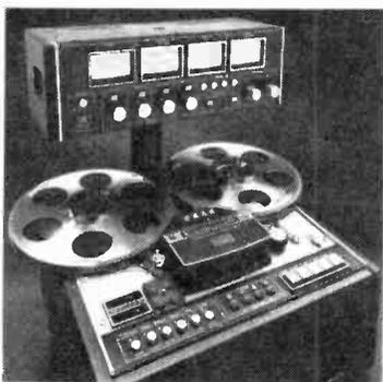
▲ **DOKORDER** redesigned 1140 4-channel tape deck has automatic multi sync/source feature, utilizing sophisticated logic circuitry.
