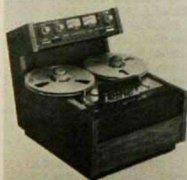
Otari Mark II professional recorder, a new generation of compact decks, offers 1/4-inch 2-channel or 1/2-inch 4-channel model, both with built-in DC servo, pitch control, separate transport and electronics, interface jack for dbx or Dolby noise reduction system.
