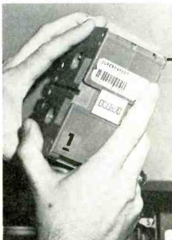
**CODED CARTRIDGE**—Perhaps a forecast of things to come is external bar code label on videotape cartridges used in RCA's TCR-100 for electronic identification of new automation accessory. Unveiled at the recent NAB in Las Vegas, the system integrates TCR-100 into a television station's technical automation system, with potential applications for radio broadcast libraries of music cartridges.
