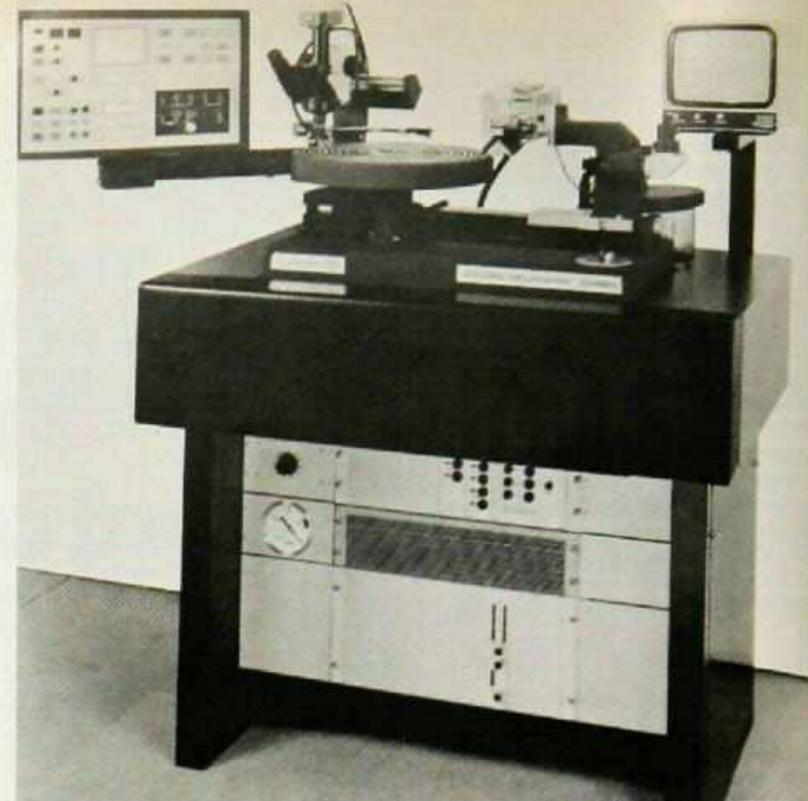
State-of-the-art: New VMS 80 Neumann lathe will be delivered to first U.S. studios this year by Gotham Audio, with features including new micro-computer control panel, left, and tv monitor linked to fiber-optic groove inspection microscope.
