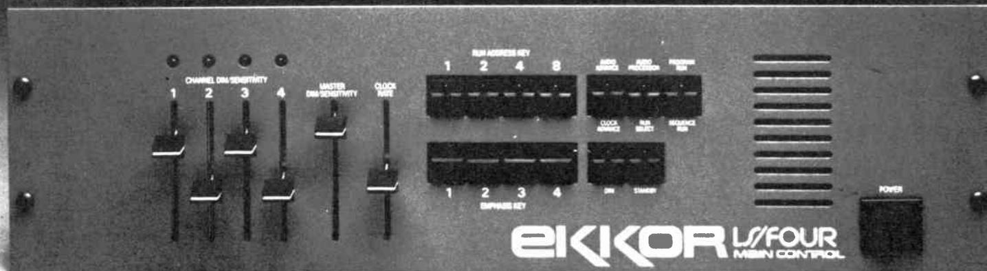
When you include the LS/Four System Light Controller by Ekkor in your entertainment lighting display, you avoid the constraints of fixed-channel controllers.
