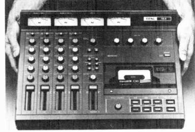
Creative Audio: View of TEAC Tascam's new Portastudio M-144. Self-contained and measuring 15-inches by 18-inches, the new multi-channel format allows the user to record basic tracks, overdub in sync and remix to stereoall on standard cassette tape.
