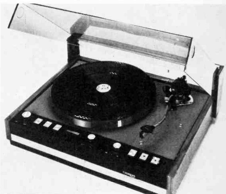
**SEMI-PRO TRANSCRIPTION**—The TD126MkIII turntable from Thorens features a servo-controlled electronic belt-drive system with DC motor and an Isotrack low-mass tonearm. The platter and tonearm are both mounted on a secondary chassis, which is suspended from the main chassis carrying the motor. Automatic pitch control compensates for any deviation from nominal speed caused by a dust cleaning arm or other differential.
