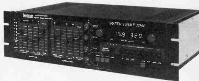
**PRIME TIME**—Lexicon's user-programmable audio processor with memory is called the Model 97 Super Prime Time. It stores eight factory-preset programs and 32 user-created programs and allows convenient off-loading of user programs to ordinary audio cassettes. The eight built-in effects include chorusing, short and long echo and resonant flanging. Dynamic Recirculation control makes it possible to achieve long delay time feedback effects. The company is located in Waltham, Mass.
