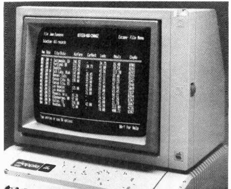
Apple Computer's new monochrome 12-inch video display monitor displays 24 80-character lines with high resolution graphics in P31 green phosphor. The monitor also has a tilt mechanism. The U.S. suggested retail price is \$229 and includes a 90-day warranty.
