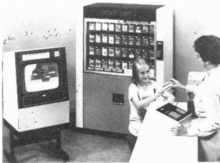
Vertx's latest electronic merchandising system is the VTV Network, which enables customers to view and select products of interest and see a demonstration on the video display monitor. The Computer Clerk terminal produces an encoded magnetic card which the customer inserts into the product dispensing machine.
