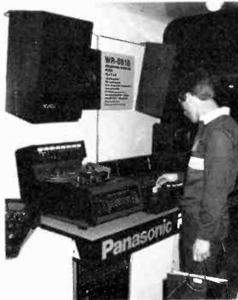
**MODULAR DESIGN**—A NAMM show browser tests a mix on the WR-8816 modular recording mixer from Panasonic's RAMSA division, being demonstrated here with Otari's streamlined MX5050 eight-track recorder. The mixer allows monitoring on all 16 input channels, and has two effect sends and two monitor sends, among other goodies in its "16 by 4 by 2" input/output configuration.
