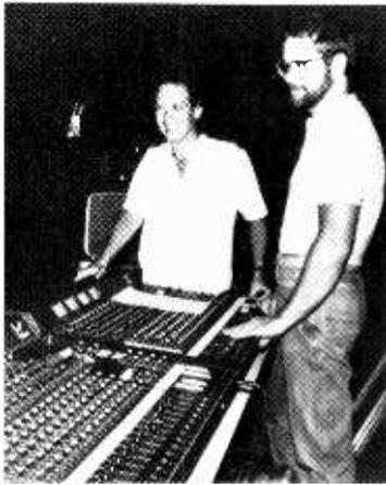
**FENDER PRO**—Lee Ritenour's current concert tour is mixed and monitored almost exclusively by Fender pro audio gear. Ritenour, left, and engineer Don Murray stand next to their Fender 4216 consoles, which feed signals to the 2244 power amps, which power the Fender 2842 wedge monitors. Other Fender components include D and P series microphones for vocal and instrument miking.
