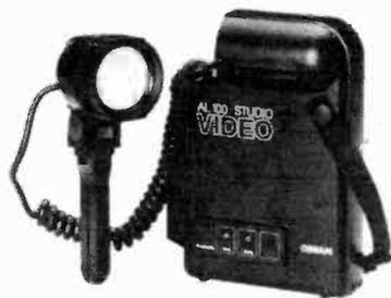
Osram Sales Corp.'s new AL 100 video light is a compact, lightweight, self-contained battery, charger and lamp head weighing in at about four and a half pounds. Angle of illumination can be adjusted from a 30 degree spot to 70 degrees wide, and the AL 100 features a 75-watt, 12-volt tungsten-halogen lamp. Contact Osram in Newburgh, N.Y.
