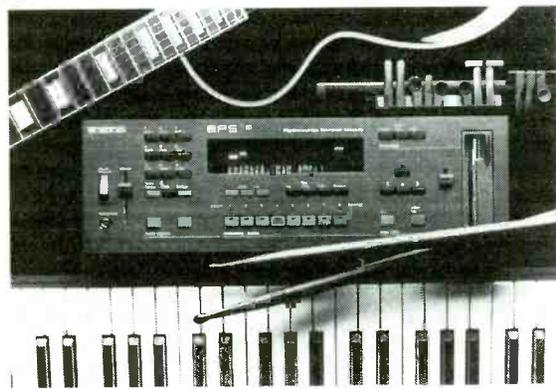
Ensoniq's new EPS-M is a rack-mountable version of the company's 16-bit variable-sampling-rate Performance Sampler. Features include the ability to play while loading disks, access to up to eight instrument sounds simultaneously, and stacking of two or more instruments together instantly. Contact Ensoniq at 609-386-7007.
