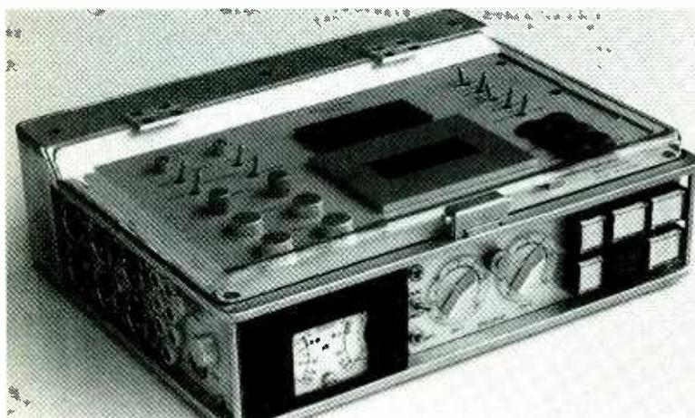
**Swiss DAT.** This rugged-looking portable, professional DAT machine manufactured by Stellavox is the first DAT deck from Switzerland. It offers a number of interesting features, including an incorporated mixer option for up to four microphones; a hefty 10-hour battery life; and climate-control mechanisms to handle difficult weather conditions. Contact Stellavox at 038-244400 in Neuchatel, Switzerland.
