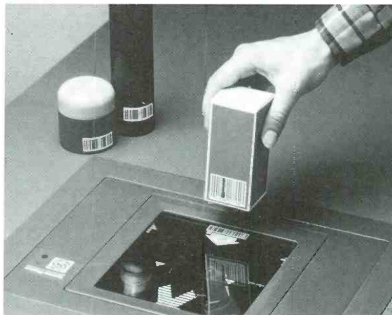
Check This One Out. Checkpoint provides electronic circuit deactivation via the Spectra-Physics Freedom Scanner.
