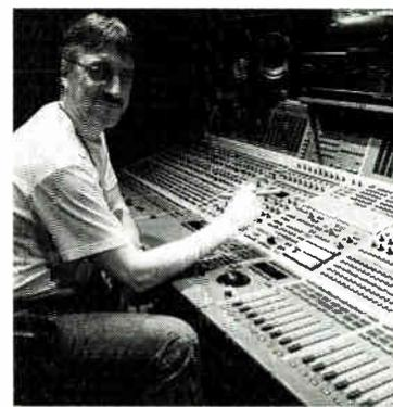
Producer/engineer Frank Filipetti is shown mixing the audio portion of James Taylor’s “Live At The Beacon Theatre” DVD Video release at Right Track Studios in New York on a Neve Capricorn digital console. Not shown is the Sony 3348-HR multitrack recorder, which—like the Capricorn—operates at 24-bit resolution.
