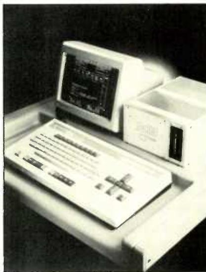
Digitor’s sync-to-tape facility allows the original soundtrack to be downloaded into the memory any number of times, but in sync with the edit decision list recorded on the floppy disk.
