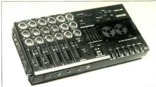
**T**he Porta 05 mixer is a 4-in/2-out design that offers plenty of versatility for both recording and playback. All four inputs accept line-level input from electronic instruments as well as standard signal processing devices. Input channels 1 and 2 also accept microphones for recording vocals or acoustic instruments or direct inputs from electronic instruments such as guitars. Trim controls are provided to set the optimum input level.
