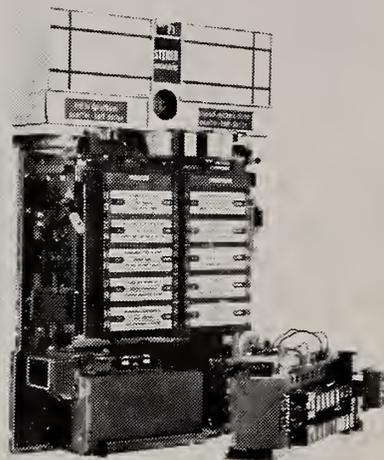
Photograph shows a Wurlitzer wallbox open for servicing. This wallbox is still operative, even though a serviceman may be working on it. If a coin has been inserted and a selection made, the box will function though the front assembly has been removed. This feature is built in all current Wurlitzer Wallboxes, with or without speakers.
