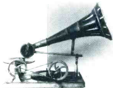
Emil Berliner's historic invention the "Gramophone," patented in 1887. The hand-cranked machine was the first to use discs—also Berliner's invention—instead of cylinders. Its success led to the foundation of the Deutsche Grammophon Gesellschaft, oldest established record manufacturing company in the world, in 1898.
