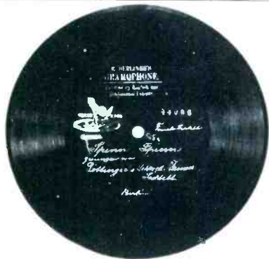
This is how the first records pressed in the Deutsche Grammophon Gesellschaft factory in Hanover looked when the company started production in 1898. The discs, with grooves on one side only, measured 17 cm (seven inches) across and the titles and artists' names were scratched on by hand. Emil Berliner's "trade marks," including the cherub inscribing a disc, were stamped on.
