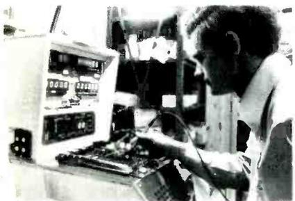
**QUALITY CONTROL** — The all-important digital scoring displays — where all eyes focus as bonus points ring up — are tested for accuracy by a Williams Electronics, Inc. technician at the firm's Chicago factory. The test is one facet of Williams' efforts to ensure quality production.
