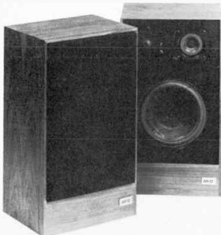
The AR-12 is an economical 3-way speaker in which the coils of the mid and high-range drivers are suspended in magnetic fluid. The fluid improves heat dissipation, allowing increased power handling ability.
