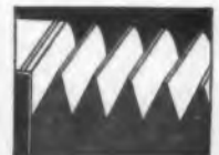
Deep fold bellows for quicker response.
