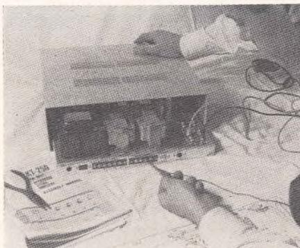
Screwdriver is used to attach speaker wires to amplifier. At right are plug cables from phonograph and FM tuner.
