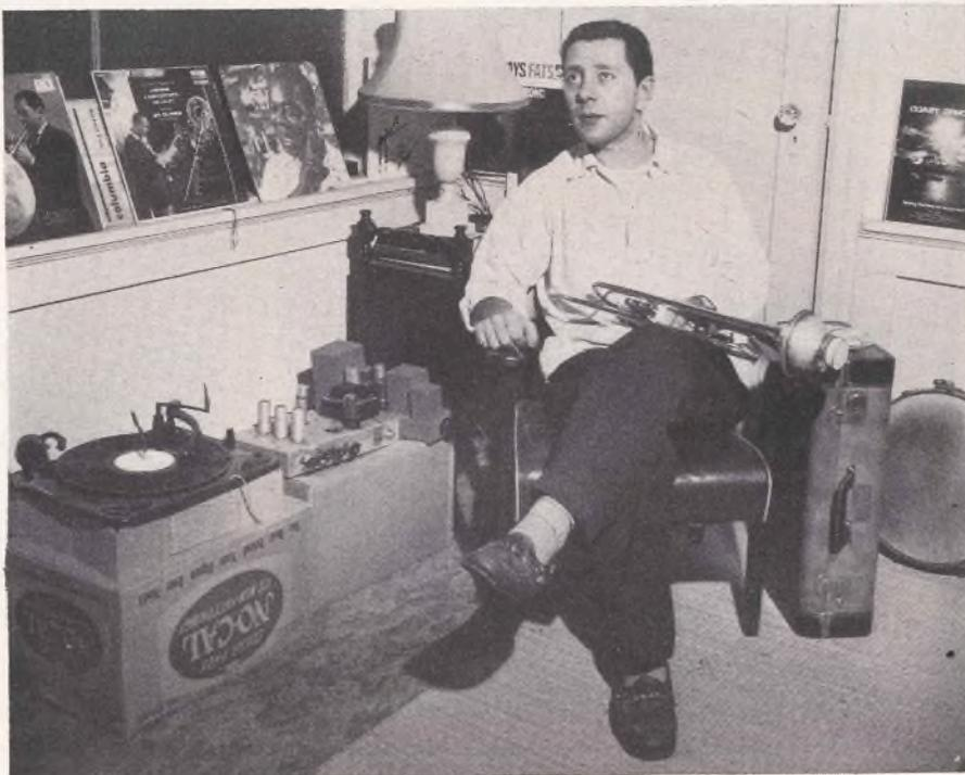
put together for him by an engineer seven years ago. His components included a Garrard record changer with a G-E magnetic pickup, a special pre-amplifier with bass and treble controls, a 10-watt Langevin broadcast type of power amplifier, and an inexpensive 12-inch speaker in a small background music baffle. The speaker and baffle were located in a recess in the wall and fed by a length of lamp cord running from the amplifier.
