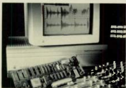
Digidesign's Sound Tools system includes a Sound Accelerator card and Sound Designer II software.
