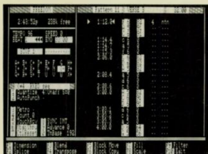
FIG. 3: The edit screen shows MIDI note on, note off, and controller values.
