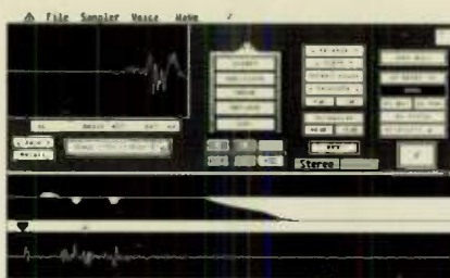
FIG. 2: A handclap sample on the Envelope page. The markers set where the claps will be truncated. The envelope (center line equals unity gain) shows a boost of a low-level section, two dips to limit some peaks, and a fadeout.
