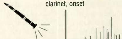
FIG. 2: The harmonic spectrum of an acoustic instrument is rarely static. Most acoustic instruments have unique onset, steady-state, and sustain spectra.
