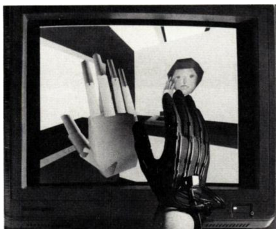
FIG. 2: With VPL's DataGlove and virtual reality system, a virtual hand will mimic the movements of a user's hand.
