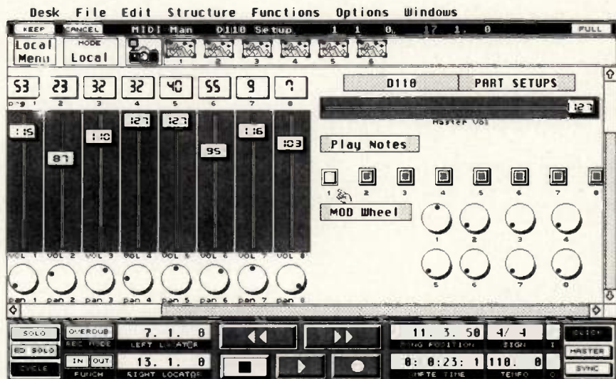
FIG. 3: Control panel built from the Cubase 2.0 MIDI Manager, controlling various part-setup parameters for a Roland D-110.
