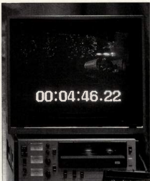
FIG. 1: "Window burn" provides an onscreen visual display of SMPTE time for easy reference during scoring.
