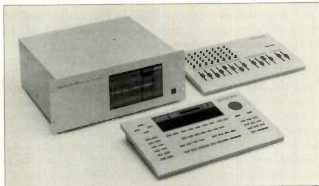
FIG. 1: The Roland DM-80 offers a complete stand-alone system for 4- or 8-track hard-disk recording.
