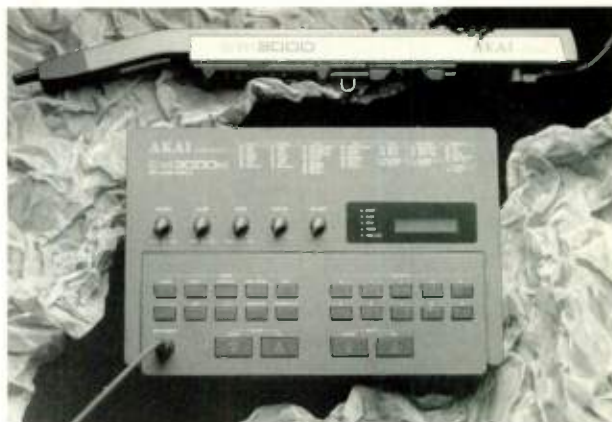
The keys on Akai's EWI 3000 wind controller don't move, responding to touch. The 3000m analog synth module (below) is monophonic.
