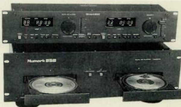
Fig. 2: As the vinyl record fades into history, CD systems such as Numark's 6020 protect the deejay's art with joy wheel cueing and tempo controls.
