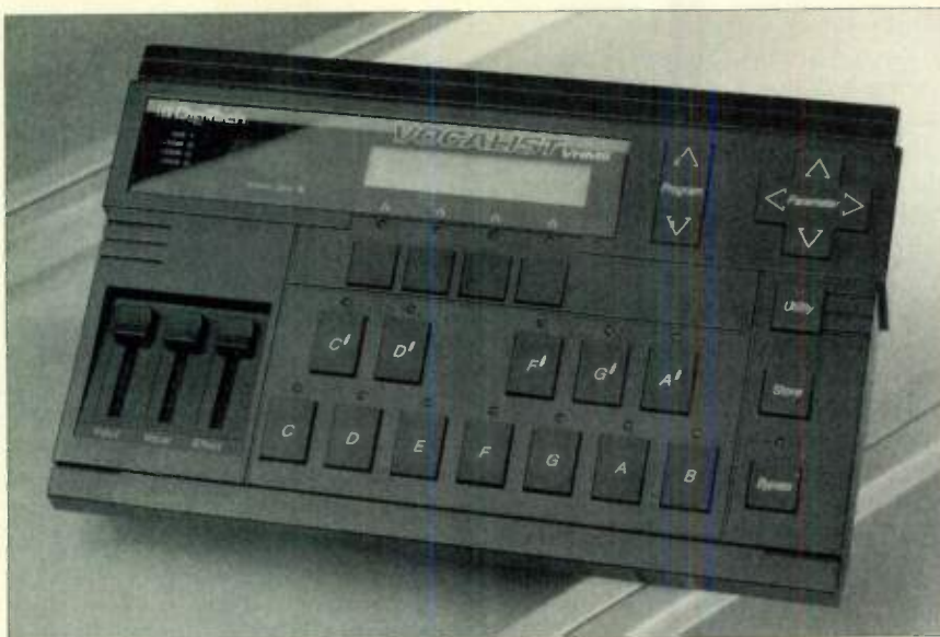
DigiTech's VHM-5 is a harmonizing device designed for vocal applications. Better known as the Vocalist, it creates four user-defined harmony notes from a monophonic audio input.
