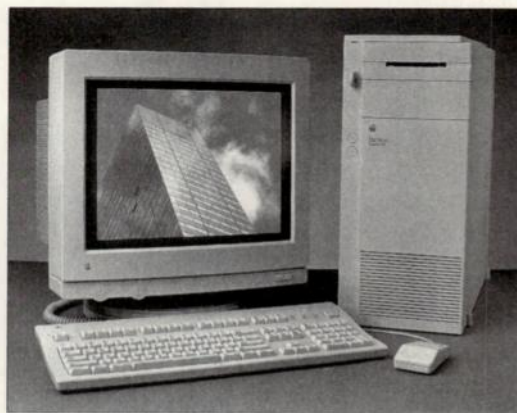
Apple's Quadra 950 offers impressive processing power but requires a Serial Switch system extension to work properly with MIDI.
