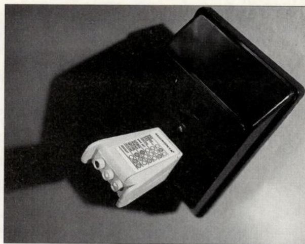
FIG. 1: Three-prong AC outlet analyzers, such as this Radio Shack model, show whether an outlet's hot, neutral, and if the ground terminals are disconnected, or if the hot terminal is reverse-wired with either neutral or ground.
