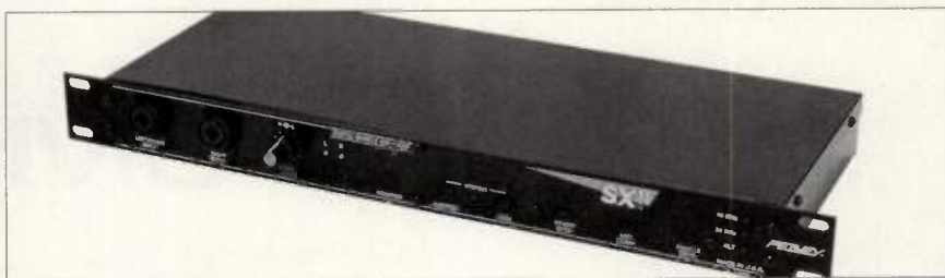
Peavey's DPM-SXII sampling module can transfer samples using SMDI in real time to the company's DPM-SP sample player.
