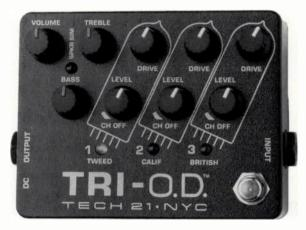
Tech 21's TRI-0.D. simulates the sound of Marshall, Fender, and MESA/Boogie amplifiers. Although the timbral controls are limited, the simulations are impressive.
