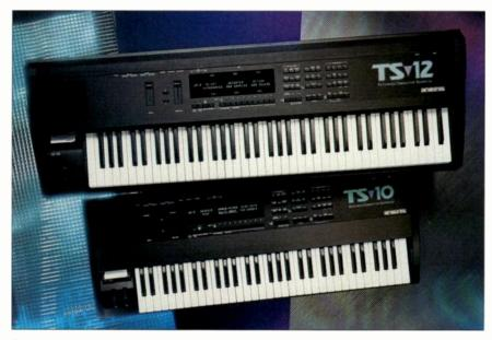
Ensoniq's twin top-of-the-line keyboard workstations offer a powerful synth, elaborate sequencer, high-quality effects processor, and the ability to play and edit EPS series and ASR-10 samples. The TS-10 (bottom) has a 61-key, unweighted action, while the TS-12 has a 76-key, weighted action.
