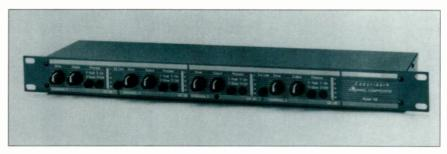
The Aphex Model 106 Easyrider compressor has four independent, mono channels that can be linked as stereo pairs. The Drive control sets both the compression ratio and the input gain. An unusual, 2-position Process switch controls the attack and release.
