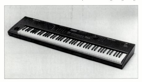
Kurzweil's PC88 combines a smooth, 88-key weighted keyboard; extensive controller functions; and 64 onboard sounds in a portable package. A optional expansion board adds a full Bank of GM sounds, supplemental sounds, and more effects.
