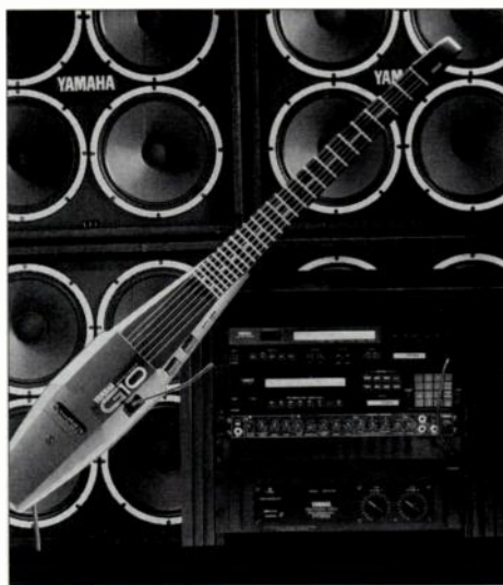
FIG. 1: The Yamaha G10 uses ultrasonic scanning to detect the vibration frequency of each string.
