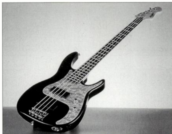
FIG. 2: The Peavey CyberBass includes detectors in each fret to determine the pitches you play.
