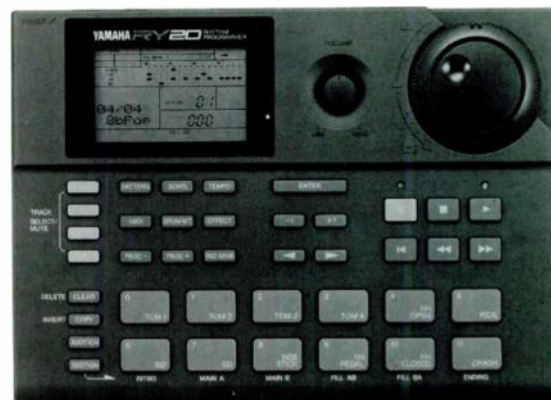
The Yamaha RY20 Rhythm Programmer provides plenty of quality sounds, a recording resolution of 96 ppqn, and a sophisticated Pattern structure.
