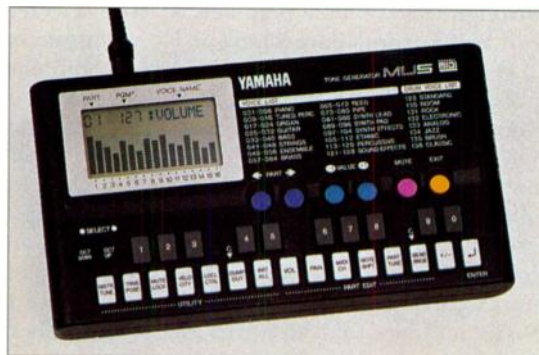
The Yamaha MU5 can be battery-powered for portability. It features 128 sounds, 28-note polyphony, and 16-part multi-timbral operation.
