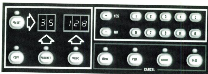
FIG. 1: Front-panel MIDI controls on the Petosa S-2000 MIDI accordion.
