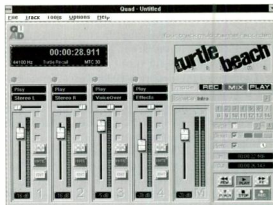
FIG. 1: Quad 's main screen is laid out much like a ministudio. Its various modes, functions, and channel settings are controlled here.
