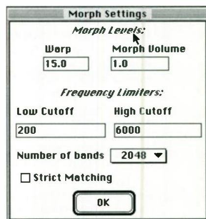
FIG. 1: SoundMorph 's Morph Settings dialog provides access to the program's few parameters. Strict Matching activates a more precise algorithm for identifying and matching harmonics.
