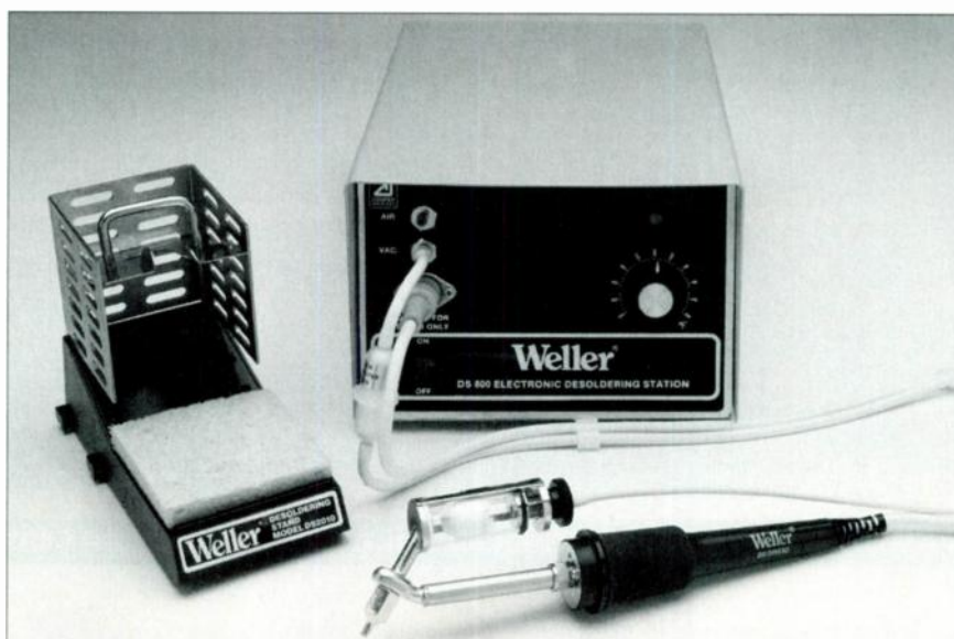
The Weller DS 800 electronic desoldering station provides a closed-loop, temperature-controlled, hollow tip through which solder is sucked into a reservoir. An internal pump provides suction.
