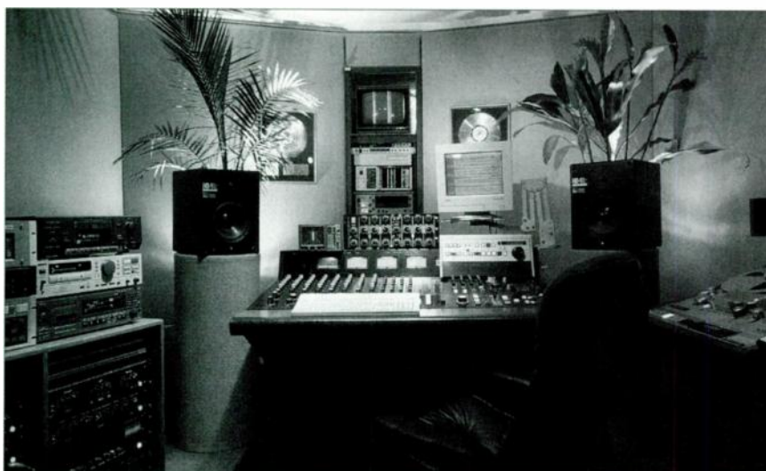
This studio includes two Meyer HD-1 near-field reference monitors on stands that isolate them from the mixer. (Photo courtesy of Rocket Lab Mastering Studios, San Francisco.)
