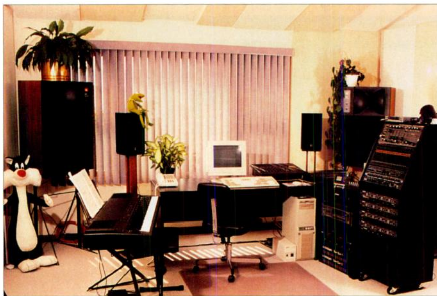
The control room includes traps on the side walls. Because there is no rear wall, additional traps are installed on the ceiling.
